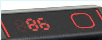
One button press on or off-load shows remaining capacity as a percentage
