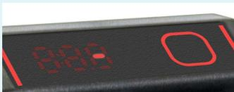
A fully discharged battery indicates as above
