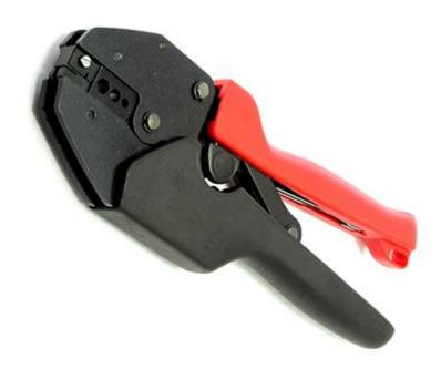
Ratchet Crimp Tool complete with die set for terminating COAX 75 ohm Micro BNC and DIN 1.0/2.3 suitable connectors to Canford group J and W broadcast cables. Die set has the following cavities:
